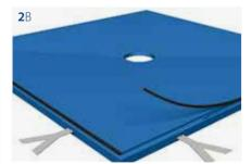
Drill two 4mm holes into the outside edges of the tray and carefully screw in the four stainless steel anchors. Stick the temporary 6mm rubber strip into the rebate of the room-facing edges of
